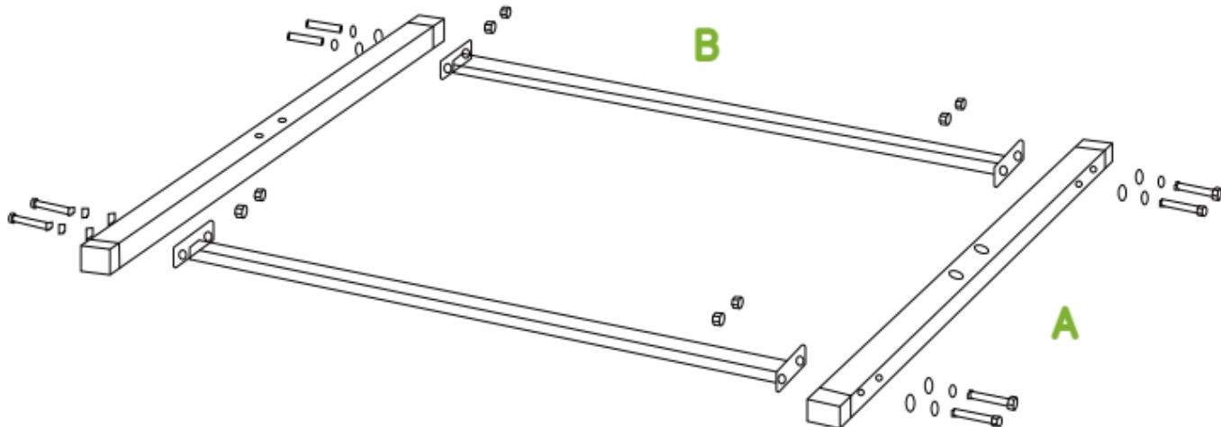
**Step 2:** Connect the TWO of the **Vertical Pipe (#C)** to the base with the following accessories: 4 x **M12 X 20 Screw (#H)**.
