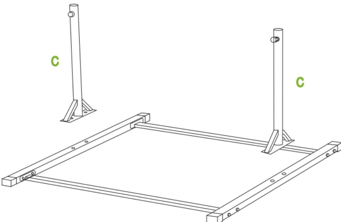
**Step 3:** Use the **Allen Wrench (#L)** and the **Small Open Spanner (#K)** to connect the **Wood Bar (#D)** with the **Adjuster Pipe (#E)**. In this step, you need 2 x **M8 X 55 Screw (#I)**.
